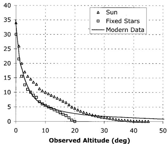
Fig. 10. Tycho's measured refraction in air.
