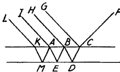
Fig. 12. Kepler's model for multiple reflections.
